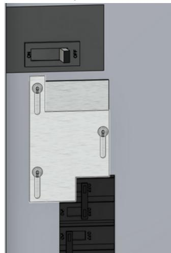
10 Test the kit to ensure that **BOTH** breakers cannot be **ON** at the same time.
