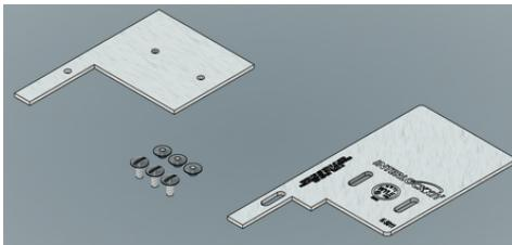
3 Temporarily attach the back plate kit using sticky tape to hold it in place and ensure a proper fit. Once in position mark the holes. Hold off on drilling holes until step 7.
