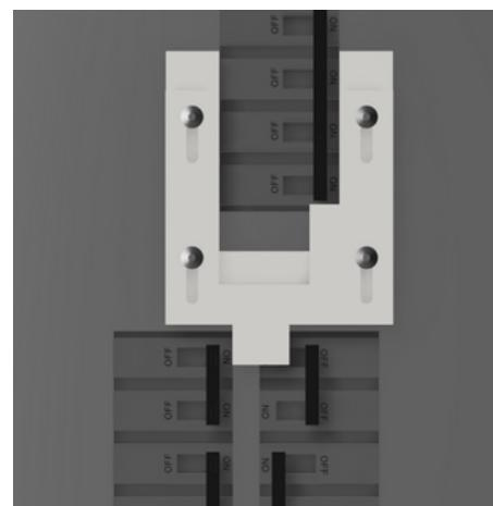
9 Set the **MAIN** and **GENERATOR** breakers in the **OFF** positions and reattach the panel cover.
