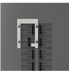
9 Set the **MAIN** and **GENERATOR** breakers in the **OFF** positions and reattach the panel cover.
