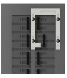
Set the **MAIN** and **GENERATOR** 9 breakers in the **OFF** positions and reattach the panel cover.
