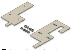
Temporarily attach the back plate kit using sticky tape to hold it in place and ensure a proper fit. Once in position mark the holes. Hold off on drilling holes until step 7.
