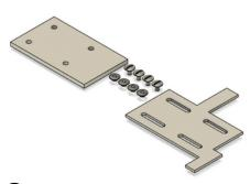
3 Temporarily attach the back plate kit using sticky tape to hold it in place and ensure a proper fit. Once in position mark the holes. Hold off on drilling holes until step 7.
