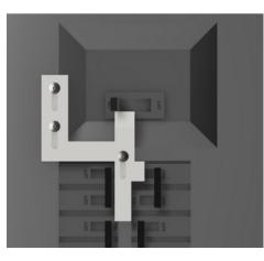
**9** Set the **MAIN** and **GENERATOR** breakers in the OFF positions and reattach the panel cover.
