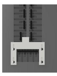
**9** Set the **MAIN** and **GENERATOR** breakers in the OFF positions and reattach the panel cover.
