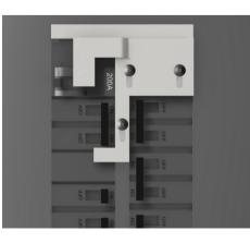
Set the MAIN and GENERATOR breakers in the OFF positions and reattach the panel cover.
