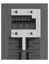
**9** Set the **MAIN** and **GENERATOR** breakers in the OFF positions and reattach the panel cover.
