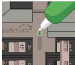
FIGURE 8 – shows Loctite application location
